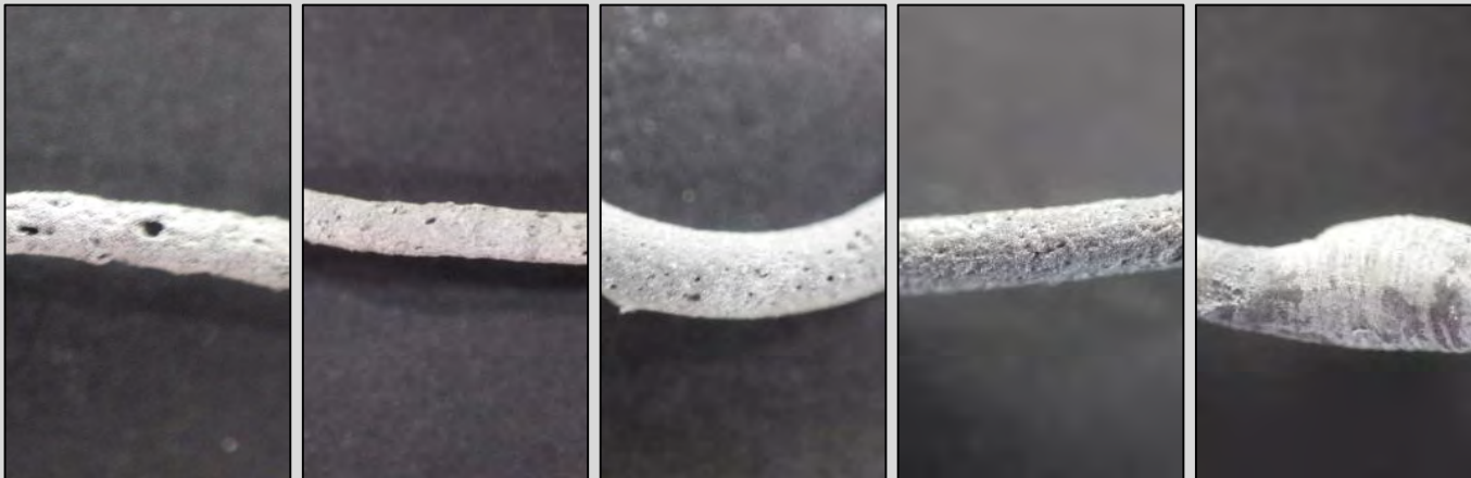
PA Route B: Extrusion Speeds from left to: 7 mm/s [0.88 mm 3 /s], 14 mm/s [1,76 mm 3 /s], 42 mm/s [5.3 mm 3 /s], 70 mm/s [8.8 mm 3 /s], 98 mm/s [12,37 mm 3 /s]
