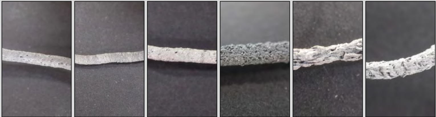
PA Route B: Temperatures extruded at 14 mm/s from left to right: 225 °C, 235 °C, 250°C, 270 °C, 280°C, 290°C
